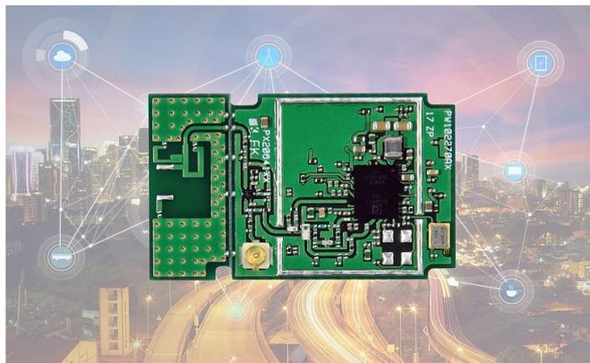
Its industrial temperature support, robust enterprise security and 802.11ac capabilities make it an ideal solution for applications like factory automation with demanding environmental conditions such as with extreme temperatures, dirt, dust, moisture, shock, and vibrations. Its low power consumption also makes it suitable for portable handheld devices.
