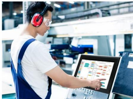
defined processes can be visualized live on the machine. ICP Deutschland offers such a 2-in-1 solution with the Cloud-based IPCs PPC-F-QGW. The series is equipped with 12 "19" displays, which have a capacitive or resistive touch. Inside, a powerful and fanless Intel® Celeron® J1900 SoC works with 4GB DDR3L SO-DIMM memory. For the transmission of the machine data common interfaces such as Dual GbE, USB as well as proven RS-232/422/485 are available.
